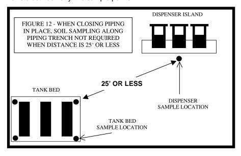
If the distance between the dispenser island sample and the nearest tank bed sample is greater than 25 feet, soil samples must be collected along the piping trench such that no
