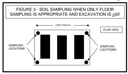
However, if the excavation is greater than 50 feet in any dimension, additional samples must be collected along each dimension of the excavation that is greater than 50 feet in length. The additional sample must be collected from the center of that dimension of the excavation as shown in Figure 4. Soil sampling must also be conducted in such a manner that no more than 50 feet exists between any two sampling points as measured along each dimension (side) of the excavation.
